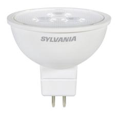
LED technology reduces energy and maintenance costs when compared to conventional light sources. They are free of UV and IR radiation minimizing discoloration and fading of materials. These lamps are rated at up to 11,000 hours life with a correlated color temperature (CCT) of 3000K. They are available with a GU5.3 base and 35° beam angle.
